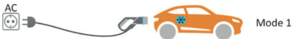
Figure 25: Charging Mode 1 (EV Charging Modes | Deltrix Chargers, n.d.).
