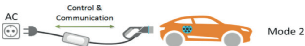
Figure 26: Charging Mode 2 (EV Charging Modes | Deltrix Chargers, n.d.).
