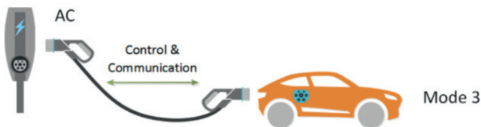
Figura 27: Modo de Carga 3 (EV Charging Modes | Deltrix Chargers, n.d.).
