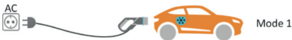
Figura 25: Modo de Carga 1 (EV Charging Modes | Deltrix Chargers, n.d.).
