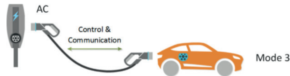
Figure 27: Charging Mode 3 (EV Charging Modes | Deltrix Chargers, n.d.).
